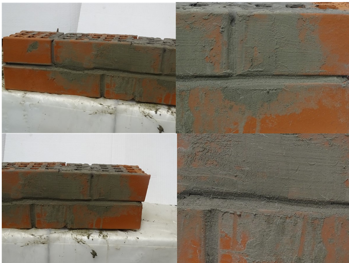
Figure 2. View of the brick wall element after structural repairs.
