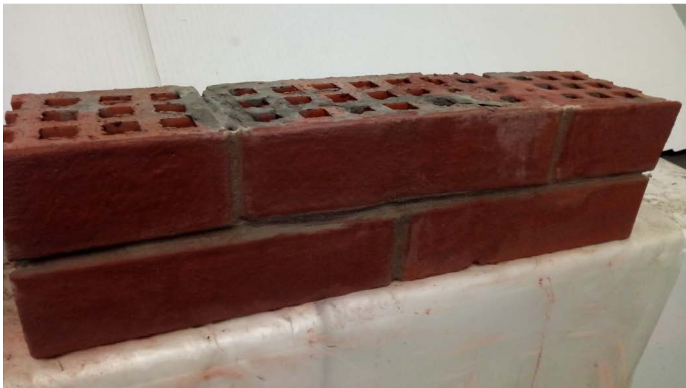
Fig. 4. The final appearance of the brick wall element after the completion of the repair with materials ARENA FORCE
