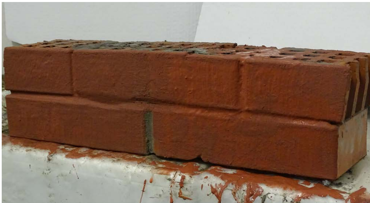
Figure 3. View of the brick wall element after applying tinted ARENA WallProtect CM.
