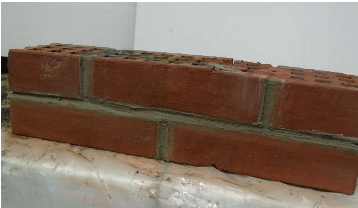
Fig. 4. The final appearance of the brick wall element after the completion of the repair with materials ARENA FORCE
